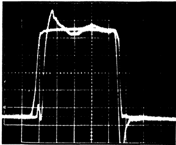
Figure 7. Switching Performance of Figure 6 Circuit, Input Pulse (left) and Output Pulse (right)
